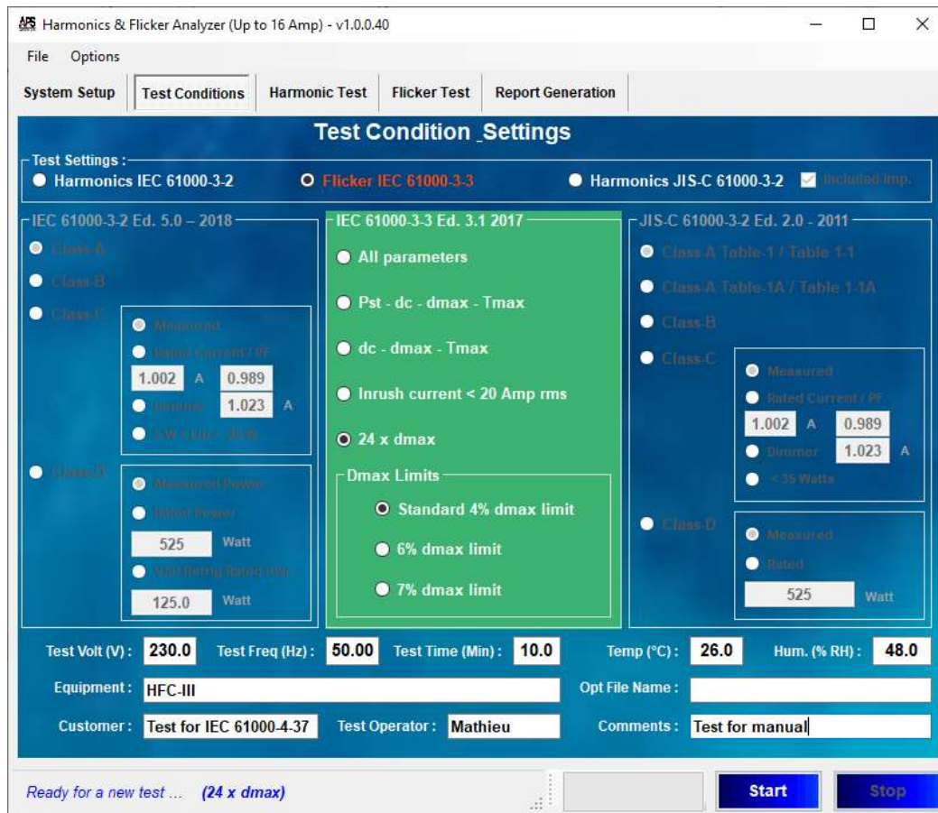
Figure 28 Selecting the “24 x dmax” test with the 4 % standard limit
