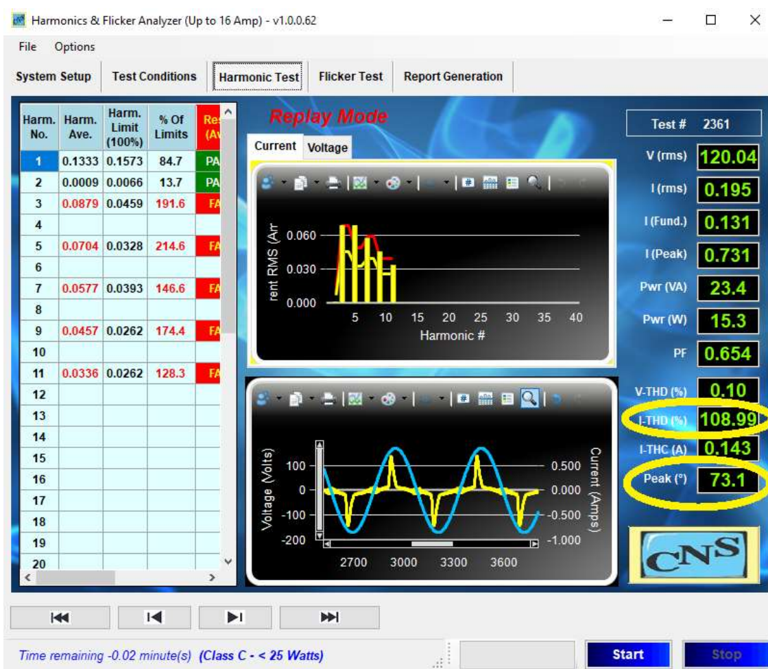
Figure 33 Lighting product < 25 Watt that fails all 3 tests per Clause 7 of IEC 61000-3-2 (2018 )
